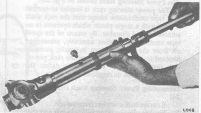
Fig. 25. Assembling rack shaft to cylinder
